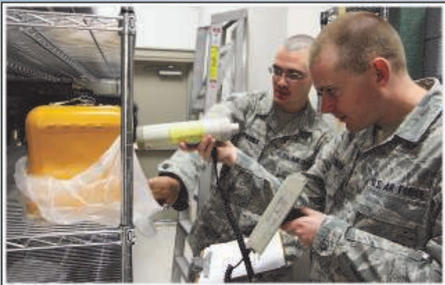
LEFT: A1C Zemanek and A1C Goodman from Bio-environmental Engineering are using an ADM-300 radiation meter to accomplish our biennial scan of a few of the artifacts in our collection. Shown is A1C Goodman scanning our WWII Gibson Girl radio. Photo: Hal Sellars
