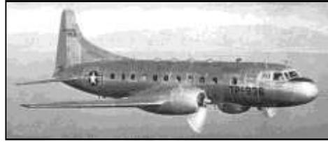
The T-29 (Model A) had fourteen fully-equipped stations for student navigators and one radio station. Each student had access to a map table, LORAN scope, altimeter and a radio compass panel. In the cabin’s roof were four astrodomes for taking celestial observations and the cabin was also equipped with four driftmeters. The aircraft was fixed with a large belly radome. The T-29A was not pressurized but was fitted with oxygen equipment. The first flight of the T-29A was on 22 September 1949.
