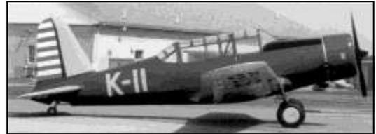
Named the "Vibrator" by the pilots who flew it, the BT-13 was powered by a Pratt & Whitney R-985 engine. But to counter the shortage of these engines early in the BT-13 production program, 1,693 Valiants were produced in 1941-42 with the Wright R-975 engine and were designated as BT-15s. By the end of World War II, over 10,000 BT-13s and BT-15s had been accepted by the Army Air Force.
