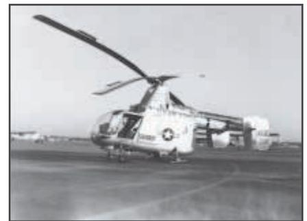
A Huskie on rescue alert could be airborne in approximately one minute. It carried two rescue men/firefighters and a fire suppression kit hanging beneath it. It often reached crashed airplanes before ground vehicles arrived. Foam from the kit plus the powerful downwash from the rotors were used to open a pathway to trapped crash victims to permit their rescue.
