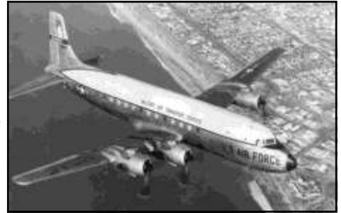
The C-118 was a direct follow-on of the earlier DC-4 model, but with a larger fuselage and more powerful engines. The C-118 was the first Military Air Transport Service’s (MATS) aircraft to fly the Atlantic Ocean non-stop. The airplane was used in many theaters throughout its long career. In 1964, C-118s were added to MATS aeromedical evacuation units in the United States. They remained in service until being replaced by the more modern jet powered Douglas C-9A Nightingale.
