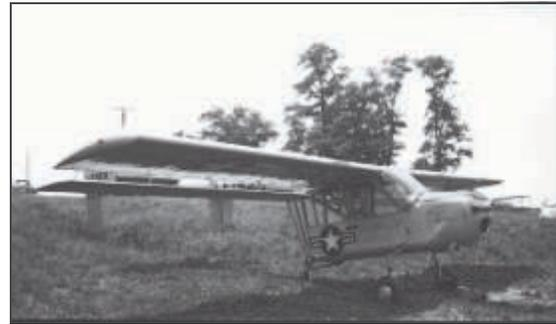
The Boeing plant at Wichita, Kansas designed the Scout for maximum visibility and good flight control at extremely low speeds. Intended for use by ground forces, it was easily dismantled and transported on an Army truck or in a C-97 transport aircraft.
