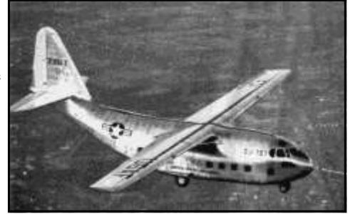
Two prototypes of the XCG-20 were built (47-786 and 47-787, pictured) with (47-786) as the first of the two chosen for conversion to power and redesignated the XC-123. The aircraft was fitted with two 1,900 hp Pratt and Whitney air cooled radial engines. As the aircraft had been designed as a glider, no provisions had been made for fuel. As a result, the fuel had to be carried externally and the rear of the engine nacelles became the fuel tanks and were designed to be jettisoned in an emergency.
