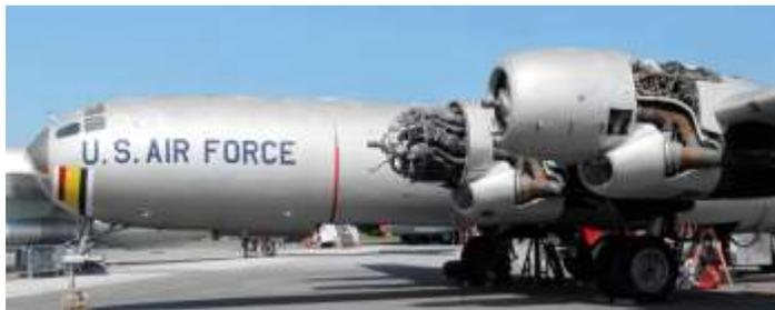
Full-time restoration work is underway on our KB-50J. Adapted as a refueler from the B-50 bomber, which in turn evolved from the B-29 of World War II, the KB-50J filled a huge void in air refueling capabilities during the early part of the Cold War.
